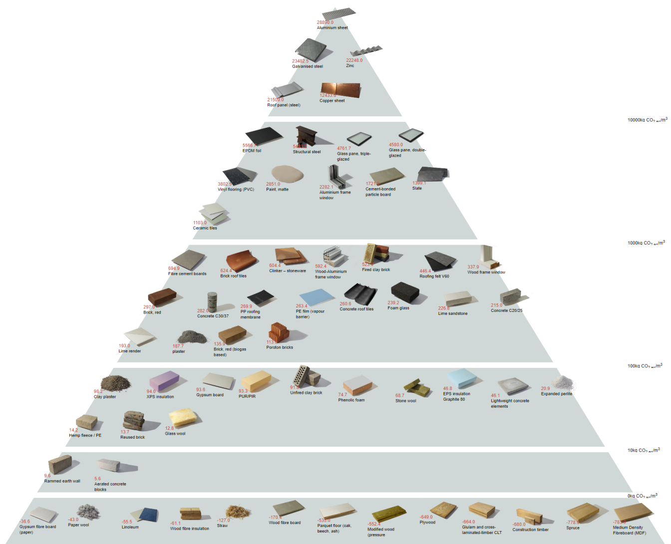
Fig 10. The Construction Material Pyramid by CINARK - Center for Industrialized Architecture, The Royal Danish Academy showing hierarchy of upfront embodied emissions of construction materials in Denmark.
